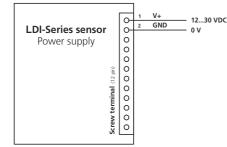
All the LDI-Series devices are overvoltage and reverse voltage protected. But for proper operation of the sensors consider the power supply requirements and the corresponding specifications.
