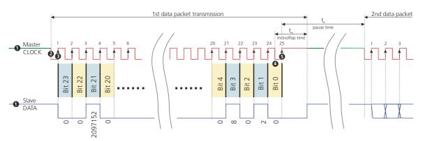
Figure 20: Timing diagram of SSI interface ( $t_m \rightarrow$  Monoflop time,  $t_p \rightarrow$  Pause time).
