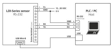
Figure 24: Connection of the RS-232 or USB interface for sensor configuration
