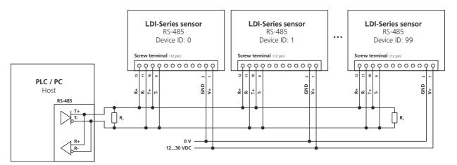
Figure 19: Connection of one or more RS-485 devices on one line,  $R_T \rightarrow$  Termination resistors
