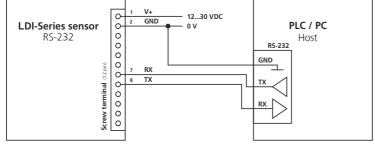
Figure 17: Connection of the RS-232 interface
