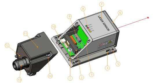
Figure 6: Sensor components with detail information
