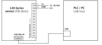
Figure 22: Connection of USB interface
