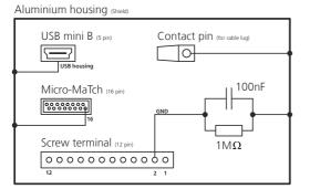
The shielding concept of the LDI-Series sensors is shown in figure 11. The aluminum housing of the sensor corresponds to shield and is also connected to the housing of the USB interface, to the Micro-MaTch connector and the shield tab. The shield tab can be used to connect the shield of a cable to the sensor shield (use an adequate receptacle).
