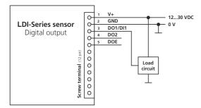
The connection to use the digital outputs of the LDI-Series laser sensors is shown in figure 14 (example with DO1, analogous for DO2 and DOE outputs).
