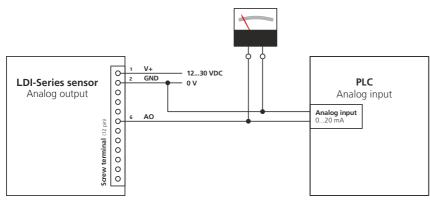
Figure 16: Connection of the analog output with a PLC (or other devices)
