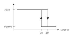
This description and diagram is correct if the ON level of the hysteresis is larger than the OFF level.
