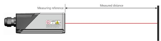
Figure 4: Standard application for measuring distances
