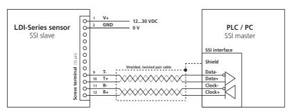
Figure 21: Connection of SSI interface with a master device
