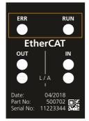
The status LED's of the EtherCAT® protocol are marked in figure 11. The possible EtherCAT® status conditions are displayed with a green and a red status LED's with three LED states – OFF, ON or FLASHING.
