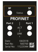
The status LED's of the PROFINET® protocol are marked in figure 9. The possible PROFINET® status conditions are displayed with two red status LED's with three LED states – OFF, ON or FLASHING.
