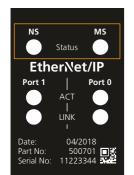
The status LED's of the EtherNet/IP™ protocol are marked in figure 10. The possible EtherNet/IP™ status conditions are displayed with two green and two red status LED's with three LED states – OFF, ON or FLASHING.
