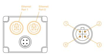
Figure 4: Connection diagram of the Ethernet port 0 & 1
