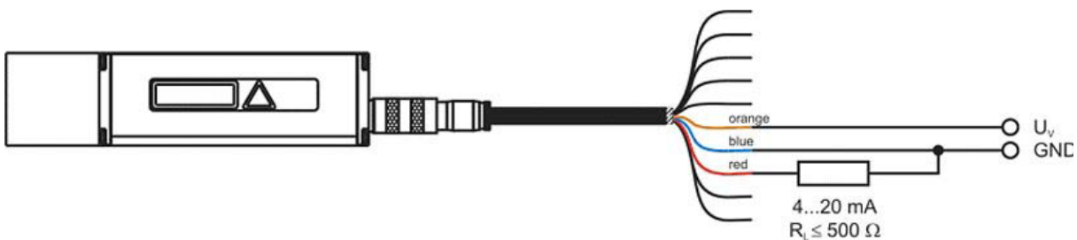
Figure 19: Wiring diagram of analog output
