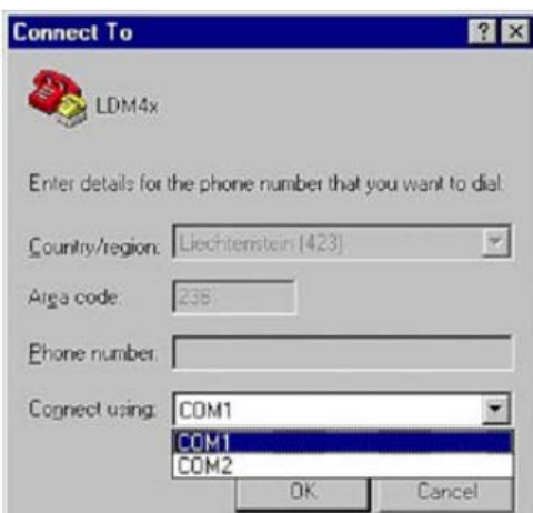
Figure 8: Establishing communication with the hyper terminal: COM port selection
