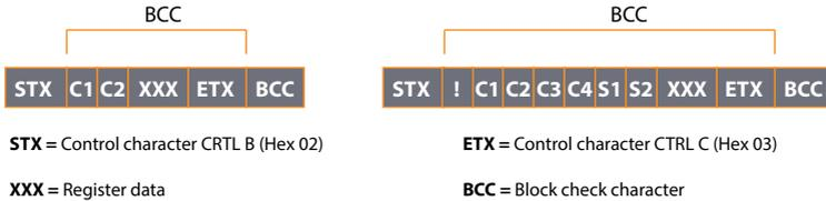
The total number of data characters „XXX“ depends on the actual numeric value of the selected data register and may also be led by a minus sign with negative values. Leading zeros are always suppressed and will not appear in the telegram. The block check character „BCC“ is generated by an Exclusive-OR over all characters between „C1“ resp. „!“ and „ETX“ (both included)
